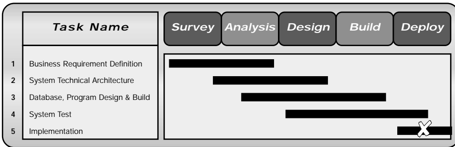
Figure 1. Failure to test for performance (X is where performance problem is discovered)
