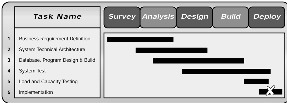
Figure 2. Inadequate Pre-deployment Performance Testing
